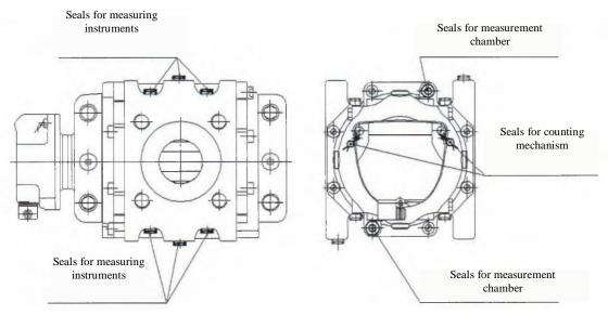
Figure 2 – Meter sealing circuit
